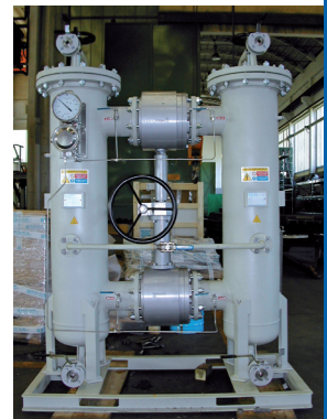
Basket duplex filter with large filtering area
