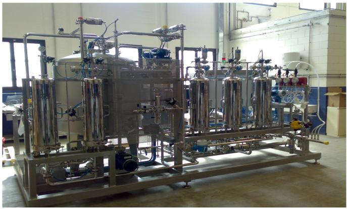
We provide pre-bottling wine The system shown includes : systems, totally filtration automated and equipped with (cleaning in CIP place), allowing sterile filtration using polyethersulphone cartridges with flow rates that can be > Chemicals dosing groups increased accordingly customer needs.
