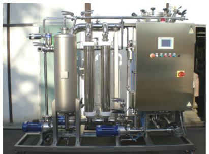
Fluxa Filtri provides tangential filtration systems using polymeric hollow fibre membranes. The automatic or semi-automatic system is used both for standard and sparkling wines, and allows the removal of yeast and the suspended solids without interfering with, or altering, the organoleptic qualities and aspects of the treated products. The field of use for this type of installation ranges from 2.500 l/h up to 10.000 l/h and beyond.
