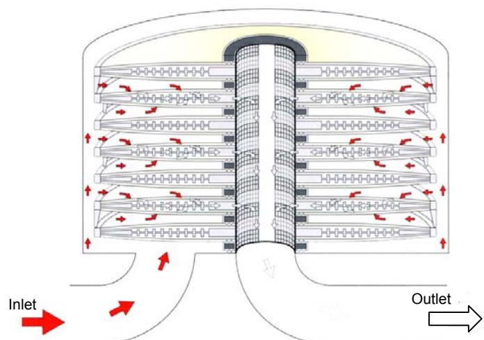
BECODISC® closed system flow diagram
