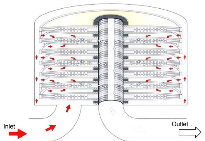
*BECODISC® closed system flow diagram*
