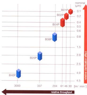
Conditions:  $\Delta p = 100 \text{ kPa}$  (1 bar), medium: water at 20 °C
