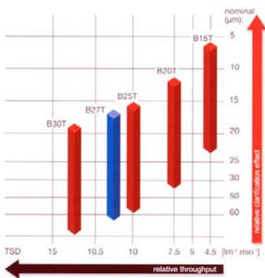
Conditions:  $\Delta p = 100 \text{ kPa}$  (1 bar), medium: water at 20 °C
