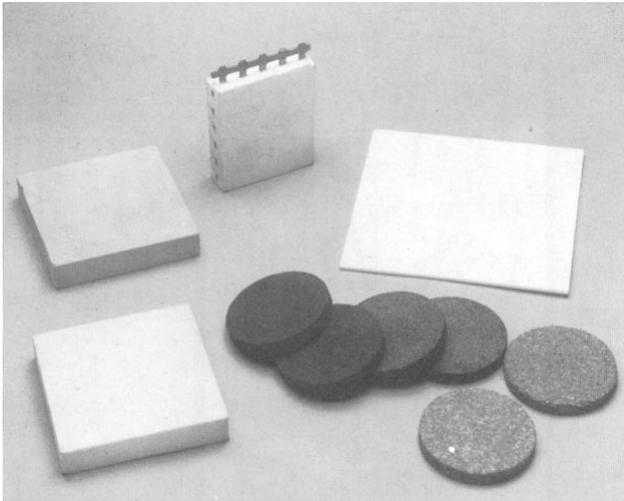
Schumacher is the most important world producer of porous materials: ceramic, plastic, graphite, activated carbon and PTFE. These are supplied as tiles or as bands.
